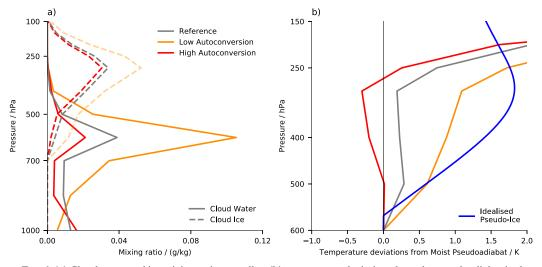
FIG. 6. (a) Cloud water and ice mixing ratio, as well as (b) temperature deviations from the pseudoadiabat in the autoconversion experiments. Darker shading represents increased autoconversion and gray represents the reference experiments. (a) An average over the convecting regions (grid points above the 90th percentile of precipitable water) and (b) the tropical mean ( $20^{\circ}N-20^{\circ}S$ ). Deviations from the pseudoadiabat were calculated as in Fig. 3.
