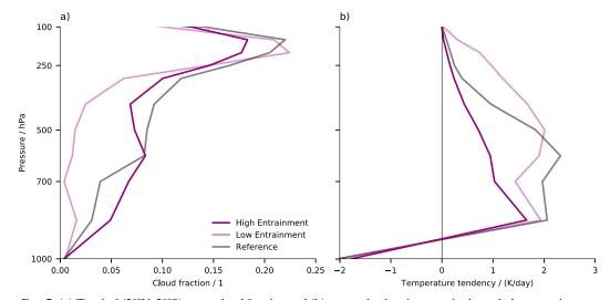
FIG. 7. (a) Tropical (20°N–20°S) mean cloud fraction and (b) convective heating rates in the turbulent entrainment experiments. Darker shading represents increased entrainment and gray represents the reference experiments.
