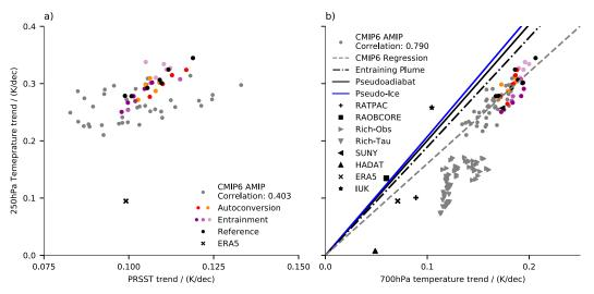
FIG. 8. Tropical (20°N–20°S) trends in (a) PRSST and (b) 700 hPa vs trends in 250 hPa temperatures for ICON perturbed physics experiments and CMIP6 AMIP simulations. Darker shading indicates increased autoconversion or entrainment as in Fig. 5. Cross-model correlation is given for CMIP6 models. Trends are calculated over the 1979–2012 period.
